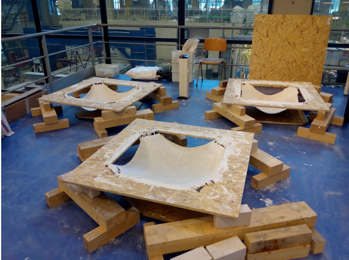
Manufacture and loading test of reinforced gypsum shells generated from hanging models – a workshop at Delft University of Technology [111].
